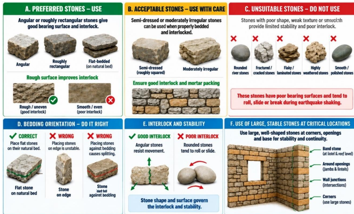
Figure 3.1. Stone selection and bedding orientation.
