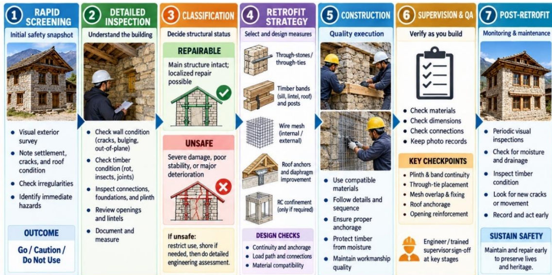
Figure 8.2. Existing building retrofit workflow.
