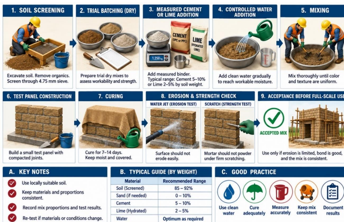
Figure 6.4. Field mortar trial and acceptance process.
